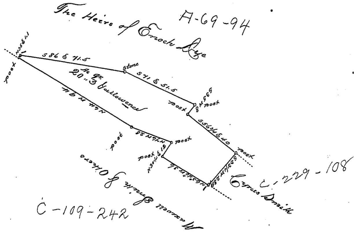
The above is a Draught of a Survey made in pursuance of a Warrant granted to Daniel Dye for 20 Ac. of unimproved land bearing date June 22<sup>d</sup> 1837 a copy of which has been sent to me for execution dated May 13<sup>th</sup> 1850, containing 20 Ac 3 <sup>9</sup>/<sub>16</sub> of allowance of six m. Cent. Situated in Canton Township Washington County Pa., Surveyed May 30<sup>th</sup> 1850.
